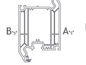
103366 115mm Open In Door Sash/Z Midrail
