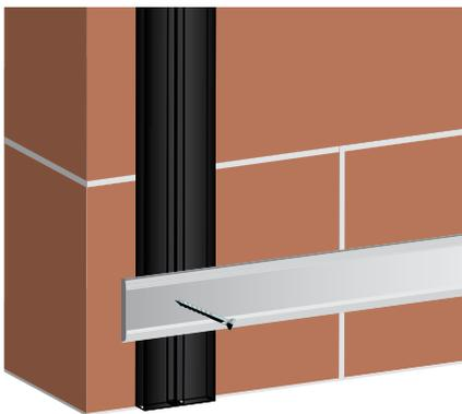
Attach a starter strip to the bottom of each joist, this will give the first cladding board something to sit on.
